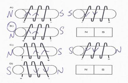
2. The electromagnets illustrated below produce magnetic fields of different intensities. The electromagnets are to be arranged in increasing order of their magnetic field.
