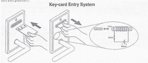
The magnetic field generated by the solenoid attracts the lock bolt when the switch is activated. This causes the lock bolt to move towards the solenoid. The hotel charged to heavier lock bolts in each key card system. As a result, the lock bolts have difficulty completing their translational motion.
