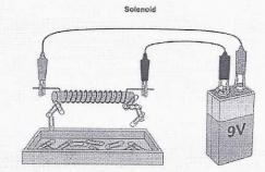
Which of the following solenoids would attract the greatest number of paper clips when connected to a 9.0 V power supply?
