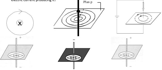
2. An electric current flows through a straight wire and produces a magnetic field.
