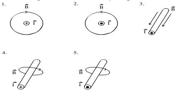
5. A magnetic compass is placed on the piece of cardboard near the wire. Which of the following diagrams shows the direction in which the compass needle will point?
